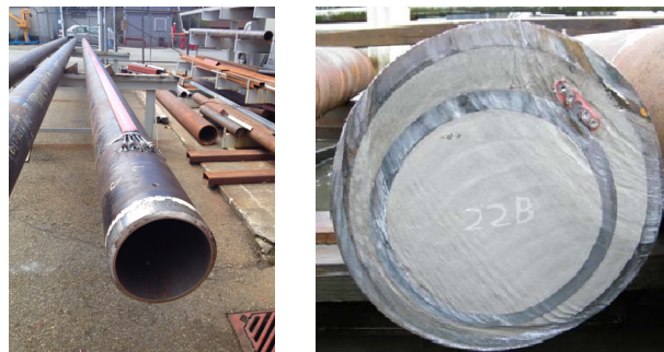
Figure 14: Full-scale tests to determine if a good seal can be obtained after P&A when tubing is left in hole: Stretching control lines at tubings during preparations (left) and cut sample with control lines cemented in place (right).
