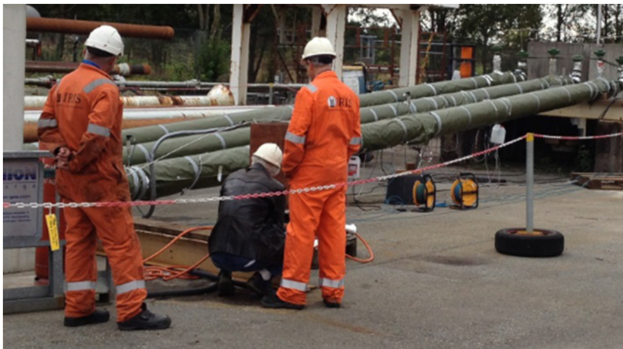
Figure 15: Full-scale assembly for «tubing left in hole» tests.
